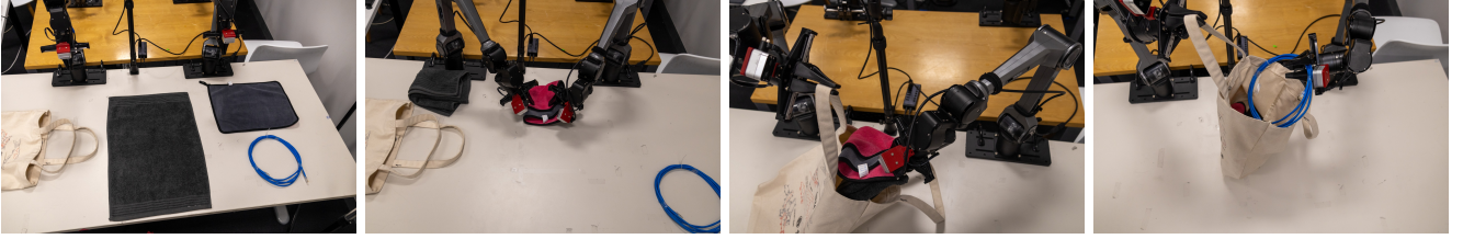
Fig. 4: Policies adapted with AutoIntervene handle deformable objects in the Towels-and-Cable Bagging task, including cloth, cables, and a tote bag.
